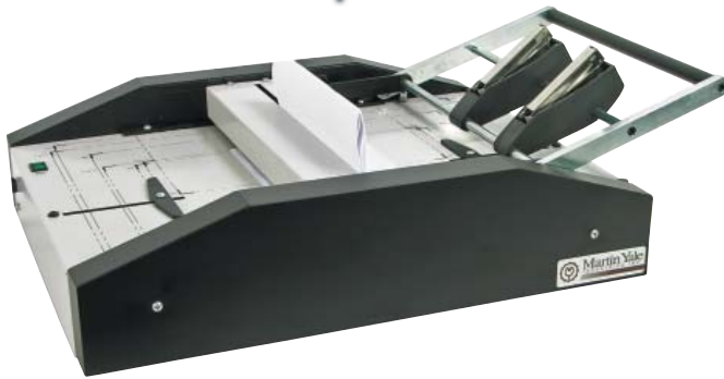
Reverse the lever to activate folder
